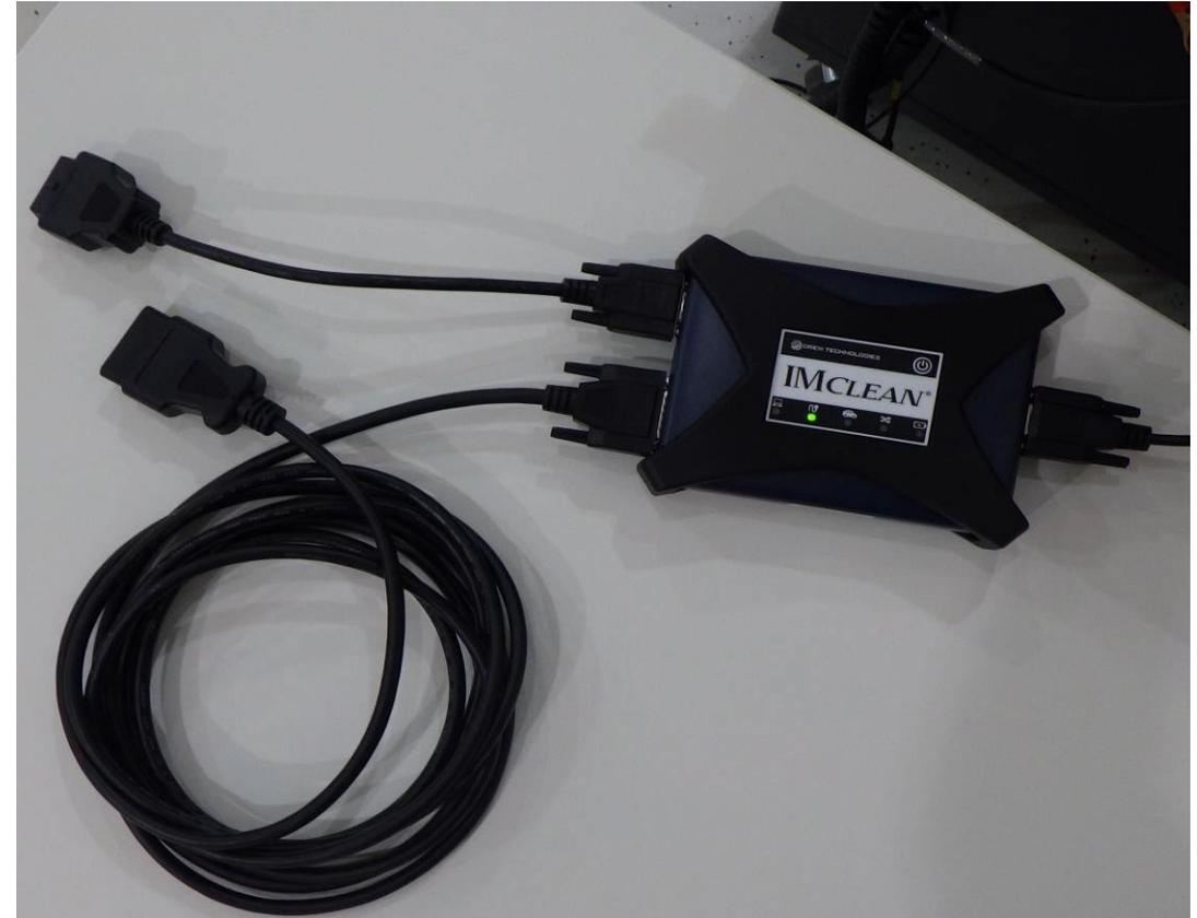
**On Board Diagnostics (OBD) Cable connected to DAD unit**
