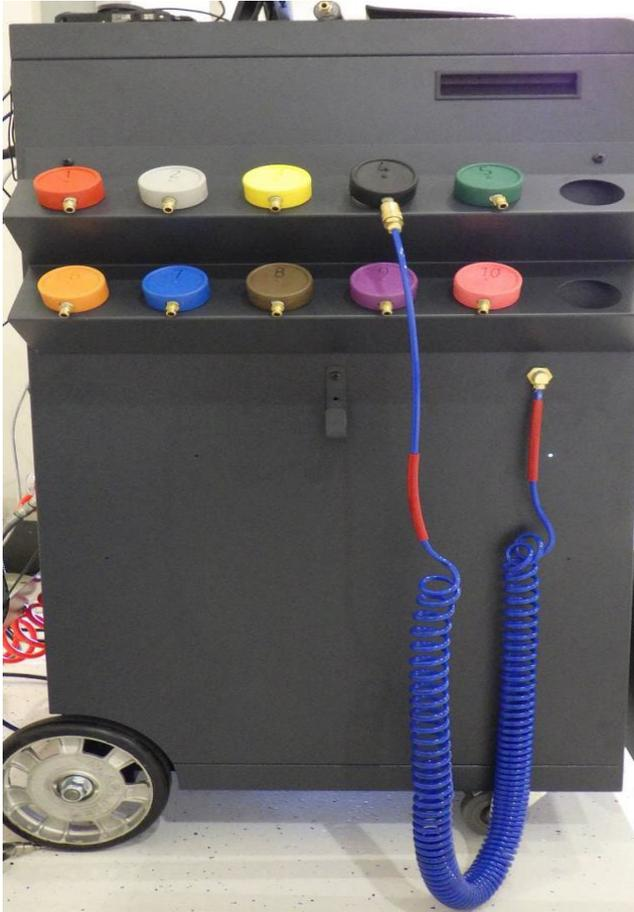
The gas cap pressure tester is located on the left side of the CDAS cabinet. This hose determines if there is a leak in the seal of the vehicle's gas cap. The adapters are for different style gas caps, although the base (black #4) adapter will fit most vehicles. If one is needed, the system will prompt you to use the recommended adapter.
