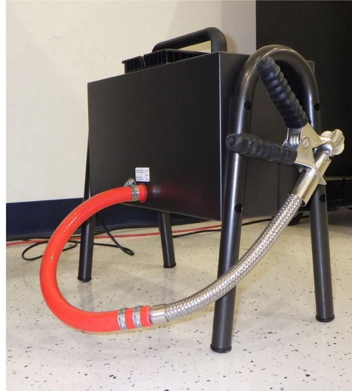
*Opacity meter and probe, for diesel inspections*
